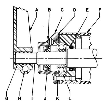
30" Units, Serial No. D-25585 and up, use the D-274-51 Roller Assembly. This Roller Assembly incorporates Oil Seals, D-235-48, back of the ball bearings used in each end of this Roller. Special tools, #TL - 1943-A and TL - 1943-B are recommended to install these Seals.
