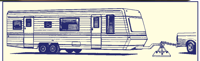
Measuring tongue weight with bathroom scale
