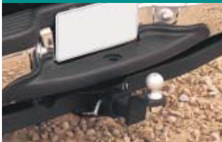
7-wire trailer wiring harness and frame-mounted hitch receiver (shown with aftermarket hitch equipment).
