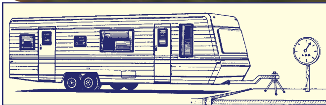
Measuring tongue weight with commercial scale
