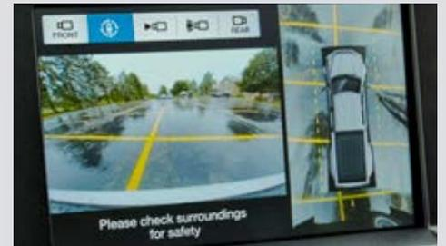
Trailer Reverse Guidance uses 3 cameras to provide multiple views of trailers, as well as steering guidance graphics, to assist with trailer manoeuvres while in reverse
