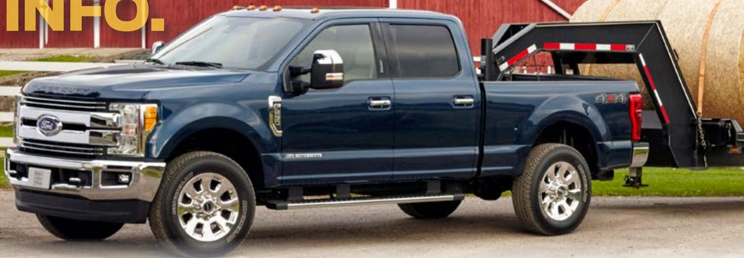
$$\text{Base Curb Weight} + \text{Cargo Weight} + \text{Passenger Weight} = \text{Gross Vehicle Weight (GVW)}$$
