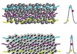
The tightly controlled 1.5  $\mu\text{m}$  diameter of Accucore Vanquish particles and the frictional forces associated with their roughened surfaces results in a tight, highly uniform packed bed that minimizes Eddy diffusion.
