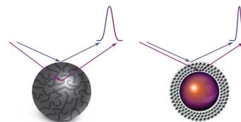
Resistance to mass transfer is minimized by the solid core design as the diffusional path of analytes is limited by the depth of the outer porous layer. The effect of this minimization is most noticeable for larger molecules.
