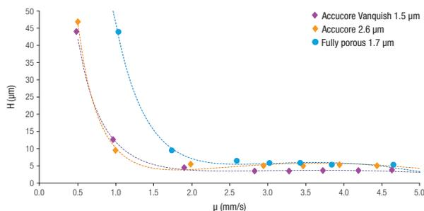
*Accucore Vanquish UHPLC columns are more efficient at optimum flow than sub-2  $\mu\text{m}$  fully porous and 2.6  $\mu\text{m}$  solid core columns. Efficiency is maintained over a wider linear velocity range.*
