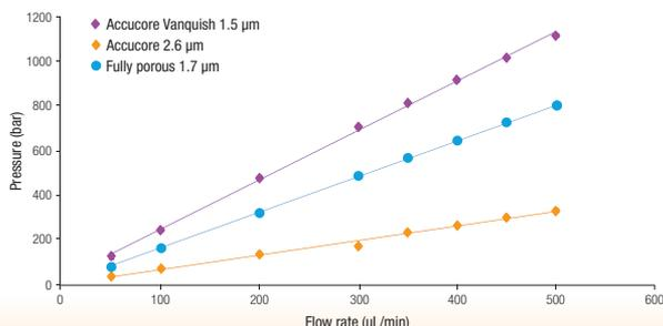
*Accucore Vanquish UHPLC columns achieve their efficiency without excessive backpressure.*
