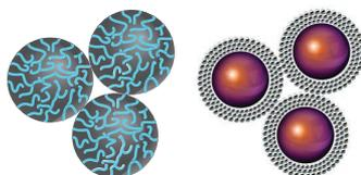
The solid core design of the particles reduces the amount of mobile phase in the column resulting in a reduced void volume and less longitudinal diffusion. This effect can be seen in the lower  $t_0$  values obtained with Accucore Vanquish UHPLC columns compared to columns of the same dimensions packed with fully porous materials.
