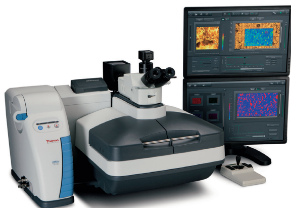
Figure 3. The modern Thermo Scientific DXR3xi Raman Imaging Microscope. This dispersive Raman system uses an Olympus microscope and is equipped with interchangeable lasers and optics enabling operations at 455, 532, 633 or 785nm.
