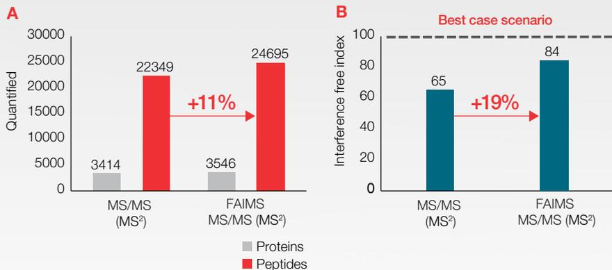
The combination of the FAIMS Pro interface, TurboTMT mode, and Precursor Fit algorithm with the Orbitrap Exploris 480 mass spectrometer enables the TMT MS<sup>2</sup> workflow to deliver TMT11plex results faster with (A) increased proteome depth and quantifiable peptides and (B) improved quantification accuracy. 1 µg of TMT11plex yeast digest standard was analyzed using a four-hour gradient.
