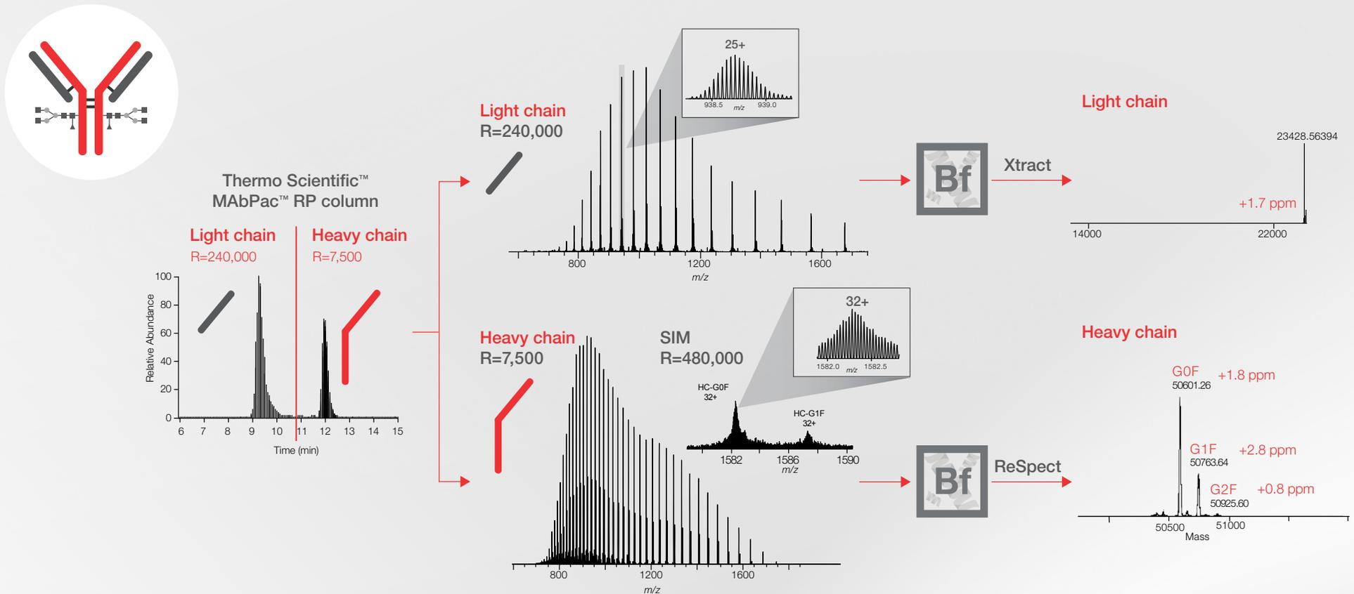
Achieving structural insights at the subdomain level are effortless. Trastuzumab was reduced, and the light and heavy chains separated by reversed-phase liquid chromatography. The light-and heavy-chain spectra obtained were deconvoluted using the BioPharma Finder software Xtract and ReSpect algorithms, respectively. Information on the heavy chain with the glycoforms was revealed, while monoisotopic masses for the light chain were also provided.
