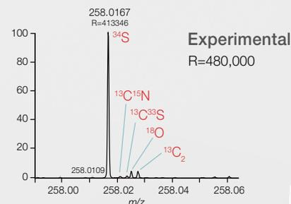
Full-scan mass spectrum of sulfathiazole, measured using the Orbitrap Exploris 480 mass spectrometer at a resolution (R) setting of 480,000 (FWHM) at *m/z* 200, demonstrates outstanding resolving power.
