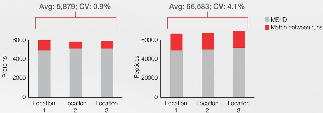
To assess instrument reproducibility, three operators at three different locations analyzed 1 µg of Thermo Scientific™ Pierce™ HeLa Protein Digest Standard (n=5). Left figure indicates the number of proteins identified at 1% false discovery rate (FDR) and the right figure shows the number of identified peptides for each of the three locations.
