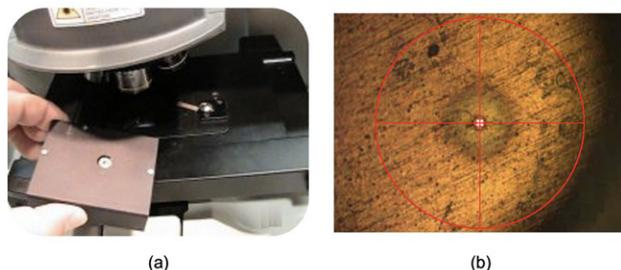
Figure 16. The alignment and calibration tool to be placed on the microscope stage (a), and the bright pinhole of the tool in the optical focus centered on the microscope eyepiece crosshair (b).
