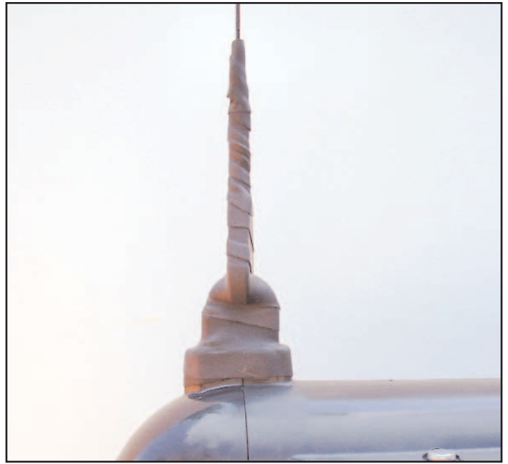
Properly installed probe using the direct connect method after application of rubberized electrical tape. Note that the tape is started at the plastic boss and wrapped upward.
