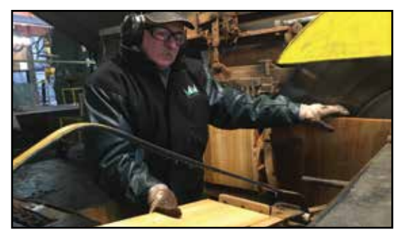
Waldun has new technology with computerized shingle machines that cut product with a much more consistent thickness than conventional machines. These machines have been a large investment for the company but as markets require thicker products, it is very important to be consistent in the thickness for the integrity and beauty of the roof.
