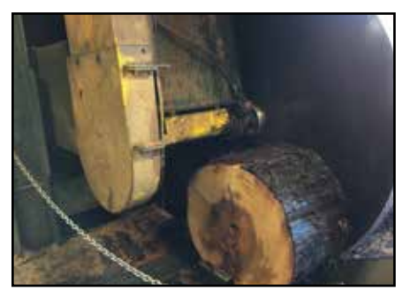
Waldun has new technology with computerized shingle machines that cut product with a much more consistent thickness than conventional machines. These machines have been a large investment for the company but as markets require thicker products, it is very important to be consistent in the thickness for the integrity and beauty of the roof.
