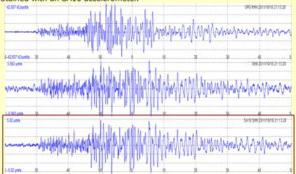
You can notice that, being P and S waves of same amplitude, the background noise of the first 10 seconds is much lower in the SA10 and also more clean in the respect of the competitor.
