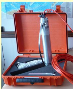
The SSBHV is a versatile multipurpose sensor solution. It finds specific application for microseism studies and noise surveys.
