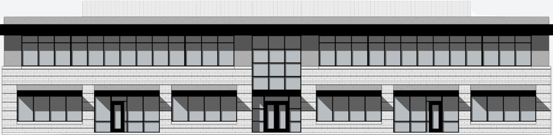
2 SOUTH ELEVATION FACING I-30 SCALE: 3/16" = 1'-0"
