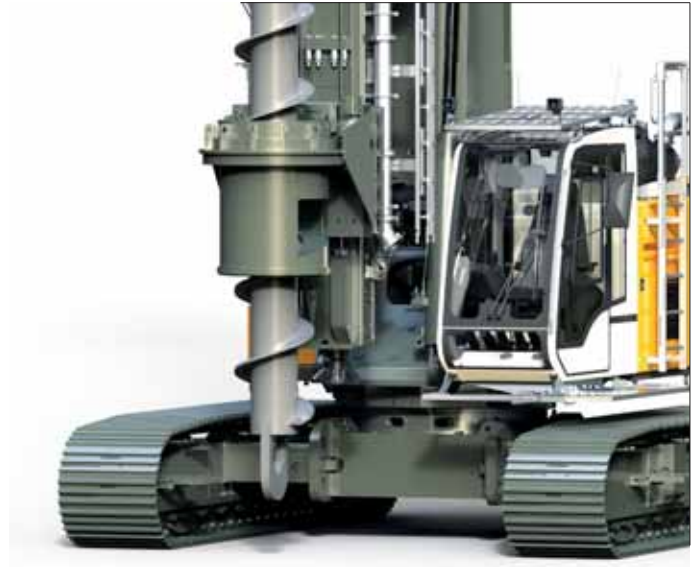
Auger with auger cleaner
