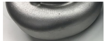
No Discernable Pattern Out of Aluminum Casting
