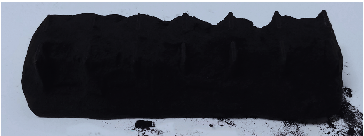
Figure 1. Example of an SLS part after the majority of bulk powder is removed.
