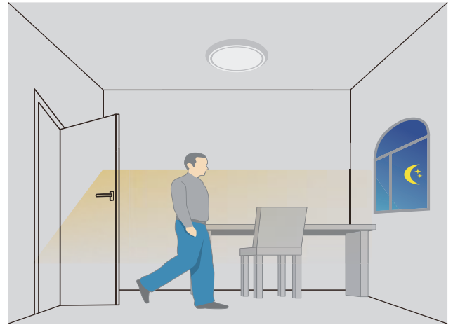
With insufficient ambient brightness, light dims to 100% when motion detected.
