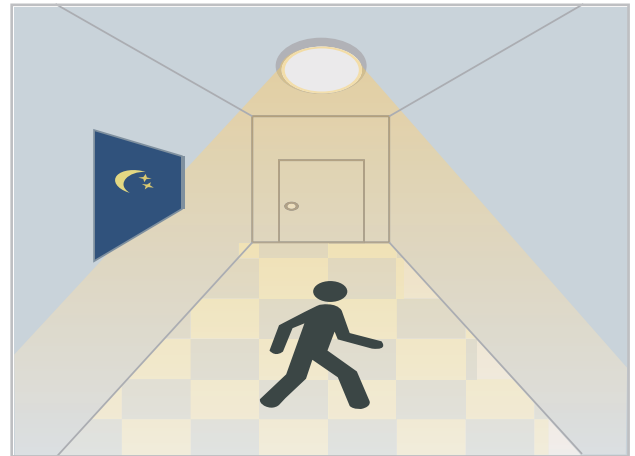
With insufficient daylight, when motion detected, light ON.
