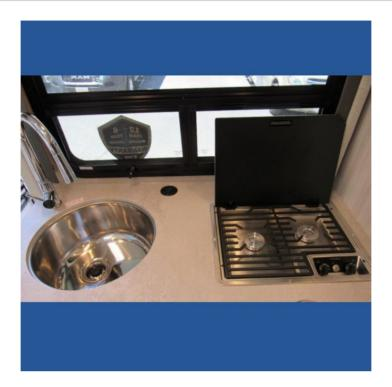
There are 2 gas burners. Make sure you lift and store the glass top on the back wall. Turn the knob of whichever burner you want to use to start/lite. Then turn the far left sparker knob clockwise. If it doesn't start right away, shut the burner off to let the gas dissipate. Then try again. Let the stove cool completely before putting the glass cover back on.
