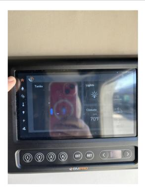
Look on the left side of the computer panel. Tap the water icon to view water settings. If using fresh water, tap to turn on the **water pump.** Tap to turn on the **tank heaters.**
