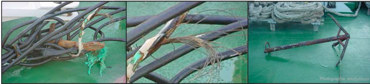
Figure 27. Cut Cable and Offending Anchor
