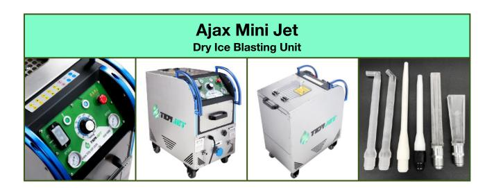
The light and size of Ajax Mini Jet is small dry ice blasting machine but the blasting power is outstanding. It is easy to use without clogging and is built with high quality. It can mill 3mm dry ice pellets into 0.6-1.2mm particles.
