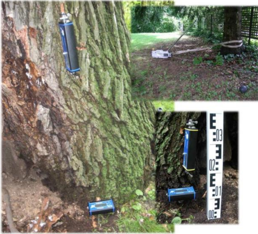
Figure A-A3: Typical tree pulling test instrument set-up. Inset details show the winch and anchor assembly (top) and elastometer/inclinometer installation (below). For illustrative purposes only; not on subject tree.
