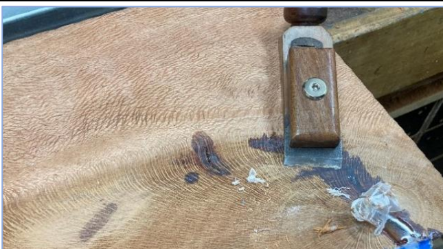
When the epoxy has set, trim off the excess. This is best done before full strength is achieved. A chisel plane is perfect for the job if you get in before the epoxy is too hard. The crack to the left of the chisel plane needs topping up with more epoxy.
