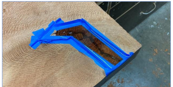
Mix the epoxy and pour it into the crack, starting at the widest part. Keep pouring slowly and work your way from one end to the other, allowing the air to bleed out as you go. Add more epoxy to create a reservoir. The epoxy will seep slowly into the crack. You may need to add more epoxy after an hour or two.
