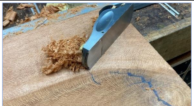
Finish off by planing and/or sanding. Planing needs to be done before the epoxy gets too hard. Repeat the filling process on the reverse side of the stock if the epoxy has not completely penetrated the crack.
