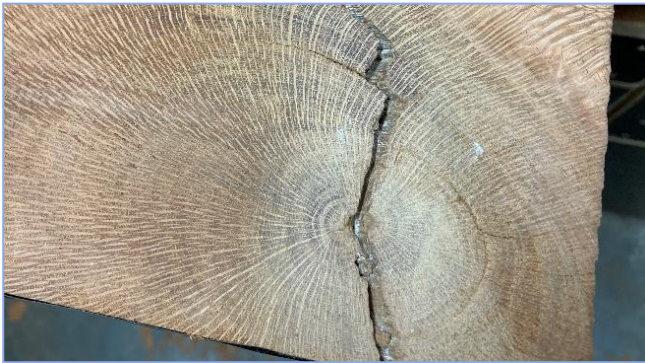
Nice piece of silky oak, if it wasn't for the big split that extends right through it! This can be epoxy filled.
