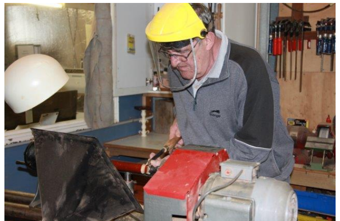
Neil McMeniman, Chair of the shed’s Workplace health and Safety Committee shows wood turners need to use a full face shield and the dust extraction system when turning.
