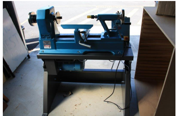
The new special tilting wood lathe for the "Blue Shed" for our restricted mobility members.
