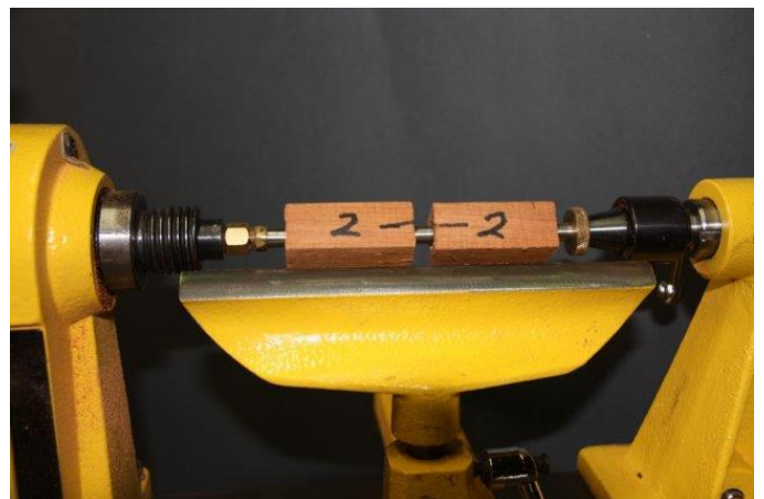
Figure 12. Load the blanks onto the mandrel with the bushes separating the blanks from each other and the ends of the lathe. You can see here how the grain continuity is matched up.
