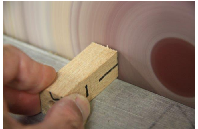
Figure 10. The next step is to square off the ends on a sanding disc so the wood is flush with the brass tube and there is a bright brass end visible.
