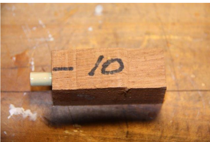
Figure 9 Now push the glue covered brass tube into the blank using a twisting action which aides spreading the glue inside the blank. Then set aside to dry for a day.
