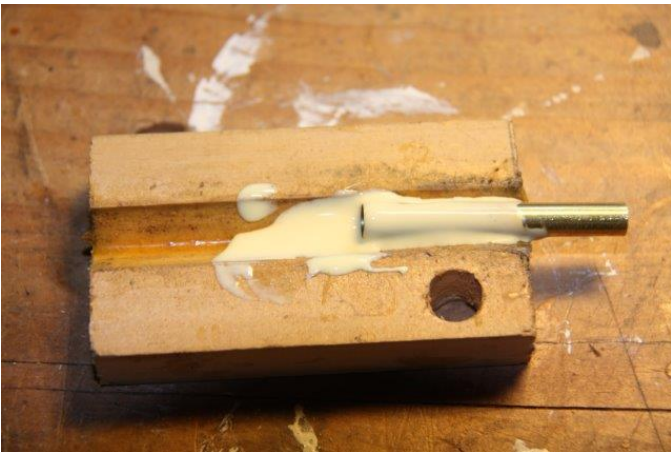
Figure 8. Glueing the tubes into the wooden blanks. Be sure to get a good coverage. This can be a messy job but a simple jig, as in the photo, helps to get both good coverage and reduce the amount of glue you get on your hands.
