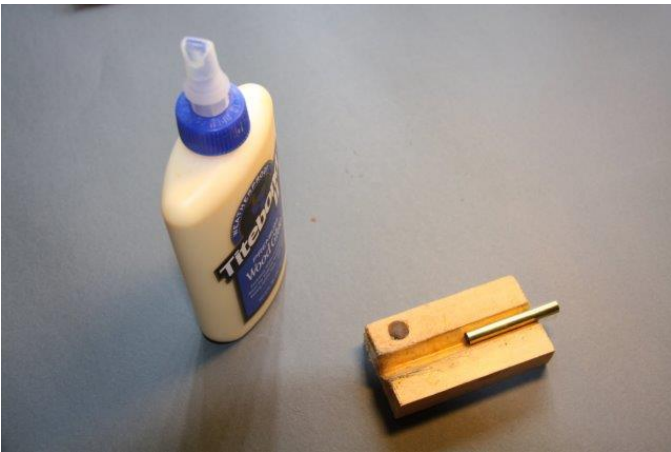
Figure 7. Take the brass tubes from the pen kit rub lightly with sandpaper and apply a quality wood working glue.
