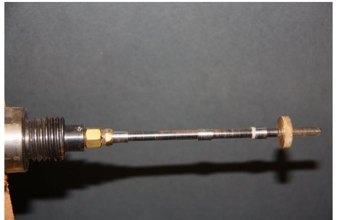
Figure 11. Now you are ready to go to the lathe where you will require a pen mandrel complete with three bushings.
