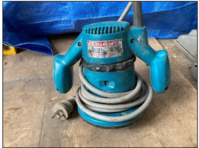
Router Makita model 3608B (1/4" collet)
