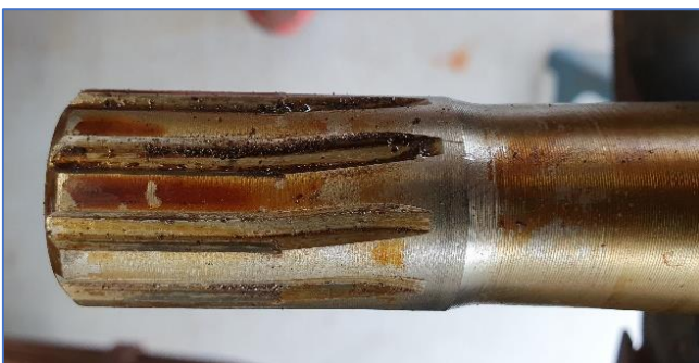
Removed shaft very close to shearing off
