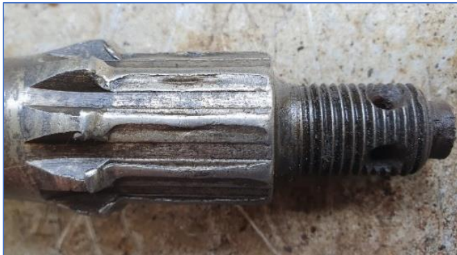
Badly Worn Front Axle Spline
