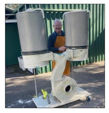
As we all know, dust is a probem in any woodworking shop, and our shed is no exception. Gavan Clark has been busy refurbishing this twin cartridge dust extraction unit, with pleated cartidge filters. These filters trap much finer dust than the needlefelt bags on some of our other filters. Gavan has also fitted big fat castor wheels to replace the skinny little ones that don't roll.
