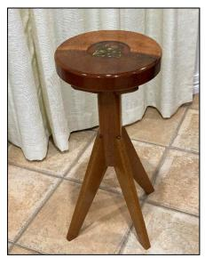
I routed a recess into the top of the stool, and the flower was set in using West's 105 epoxy, with 207 clear hardener.
