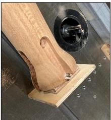
Routing mortices in the already turned legs was easy enough once I thought it through. I screwed pieces of ply to each end of the leg to provide faces to register on the router table surface and on the fence. Cutting the tenons was also quite simple using a sled on the router table.
