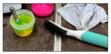
To clean a dirty cutter, soak your cutter in a cleaning solution to cut through the baked on grime. After soaking, clean off the residue.
