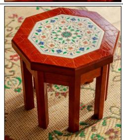
Postscript: An interesting phenomenon was observed after the coating of the tabletop with Cellulose Nitrate spray. Although various websites confirmed that one could cover shellac with cellulose nitrate, what appeared several weeks after spraying were some cracks in the shellac layer. Possibly I should have left the layer mature longer. My initial response was despondency. However, everyone who has seen it like the pattern as it gave the impression of age.
