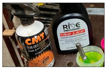
The cleaning fluid must be non-corrosive so as not to damage expensive carbide tipped cutters.
