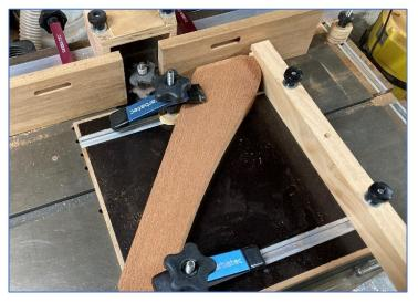
Cutting the tenons on the router table using a sled and stacked slot cutters.
