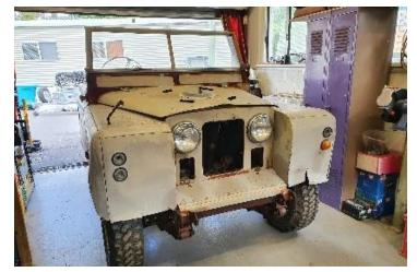
Since the last update, work to remove the remaining body panels from Ollie has proceeded. All body panels have now been taken off the vehicle apart from the firewall. Before the firewall can be removed, numerous components that attach to it on the interior side (dash, pedals, vents, windscreen, etc) and in the engine bay (steering column, master cylinders, electrical components, etc) need to be removed. This should be completed sometime next week.
