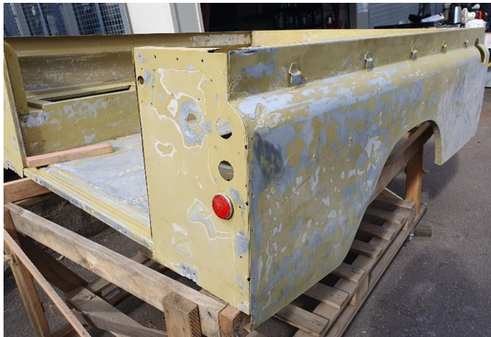
Russ' work on preparing the tub for painting
