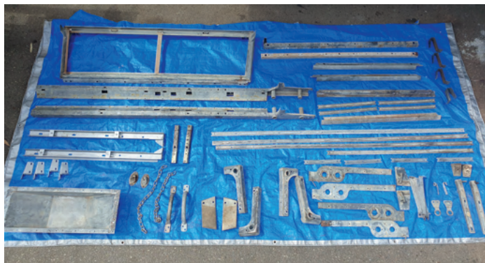
Components ready for galvanising
