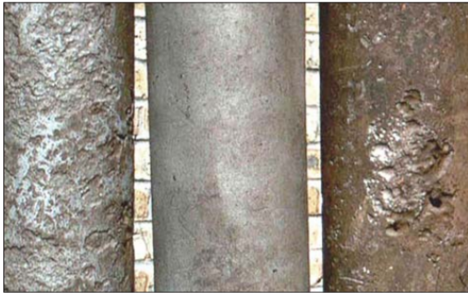
This photograph shows 6-in. (150-mm) ductile-iron pipe specimens from the Everglades, Fla., that were exhumed after an exposure of 4.25 years. The specimen in the center is polyethylene-encased pipe whereas the other two specimens are unprotected pipe.
