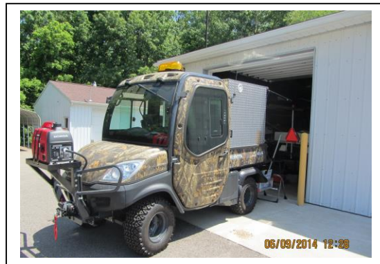
Off road CCTV Camera Vehicle
