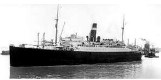
Built by Fairfield Shipbuilding and Engineering Company of Govan. She had six steam turbines driving twin screws via double reduction gearing, giving her a speed of 15 knots. 160m long 13465 tons.
