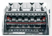
Rotary discs integral with the rotor and rings.
