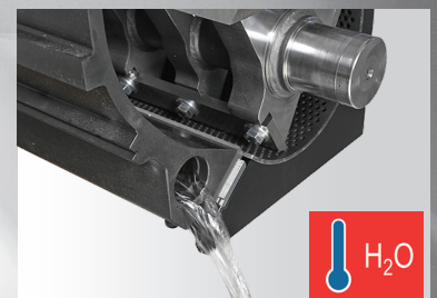
Chamber water cooling; screen equal to approximately 50% of blades rotation length.
