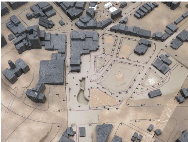
Image 2A: Wind Tunnel Study Model for the Existing Configuration
