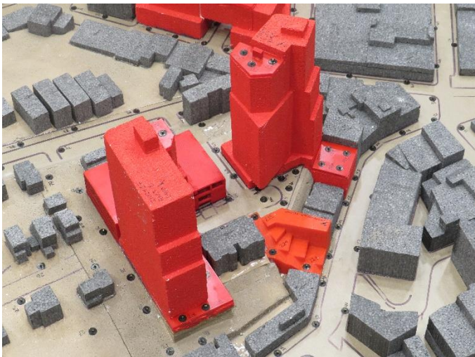
Image 2B: Wind Tunnel Study Model for the Proposed Configuration (continued from previous page)
