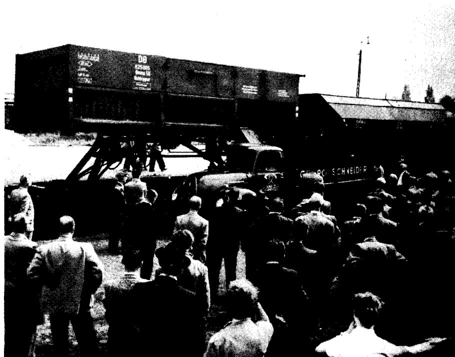
—Wide World Photo Before a group of railroad officials, a new type German hopper car shows how it unloads itself, in Darmstadt, Germany. For unloading, the hopper is automatically lifted from its understructure to the height of about 5 feet above the carriage. Then it tilts slowly to the side on which the opening is located and thus empties its contents onto the loading platform of a truck standing by. The unloading mechanism is hydraulically operated.
