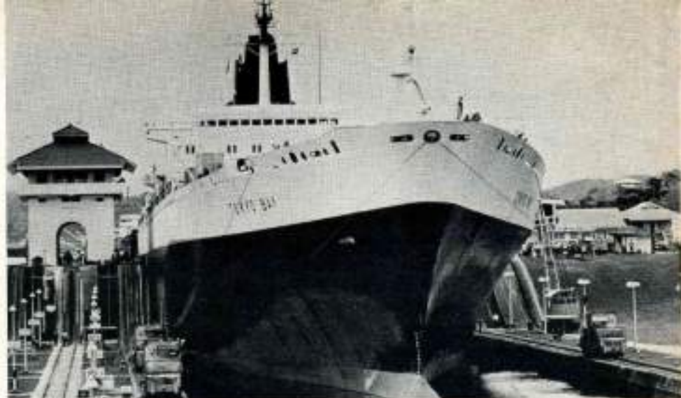
THE TOKYO BAY, shown here and on page 21 at left, the largest ship ever to transit the Panama Canal. The giant container-carrier had only two feet to spare on each side within the 110-foot-wide chambers. Panama Canal Company
