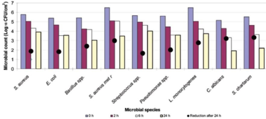
**Fig. 2. Ozone decontamination on highly polished stainless steel surfaces using the EcoQuest Breeze AT Ozone generator**
