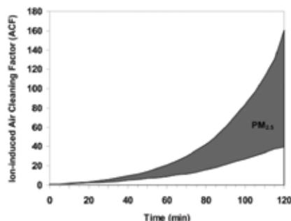
**FIGURE 3.** The ion-induced Air Cleaning Factor (ACF) for PM<sub>2.5</sub> NaCl as measured with the ELPI and integrated for different locations and orientations of the air purifier in the 24.3 m<sup>3</sup> chamber. No ventilation in the chamber. The initial PM<sub>2.5</sub> aerosol concentration =  $(0.356$ – $1.50) \times 10^5$ /cm<sup>3</sup>.
