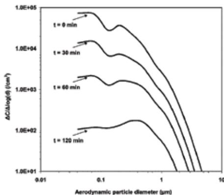
**FIGURE 2.** Particle concentration and size distribution of NaCl aerosol as measured with the ELPI in the 24.3 m<sup>3</sup> chamber with the air purifier operating facing the chamber's center at 1.7 m from the measurement point. No ventilation in the chamber. The initial total aerosol concentration =  $1.50 \times 10^5$  /cm<sup>3</sup>.
