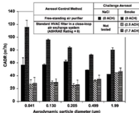
**FIGURE 4.** Clean Air Delivery Rate (CADR) determined for the NaCl and smoke aerosols as measured with the ELPI in the non-ventilated 24.3 m<sup>3</sup> chamber. The performance of the air purifier is compared to that of a standard HVAC filter (ASHRAE rating = 8) installed in the closed-loop air exchange system of the chamber.
