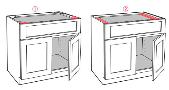
FIRST, DEPENDING ON YOUR CABINET DESIGN YOU'LL NEED TO REMOVE EITHER THE FOWARD CORNER GUSSETS ① OR LEFT AND RIGHT SIDE SUPPORTS ② FROM THE TOP OF YOUR CABINET OPENING. THIS WILL ALLOW THE SPACE NEEDED FOR YOUR SINK BOWL TO INSTALL SMOOTHLY AND WITHOUT OBSTRUCTION.
