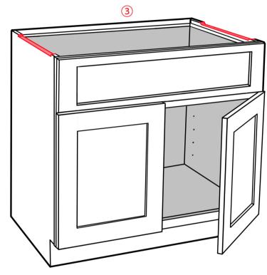
NEXT, FOR SINKS 42" AND UNDER OR WHEN USING THE SIDE OF THE CABINET AS THE ONLY SUPPORT FOR THE RIGHT AND LEFT FLANGE, THE AREA WHERE THE SINK WILL RESIDE NEEDS TO BE ROUTED DOWN 1/16" ③ SO THE SINK WILL BE FLUSH WITH THE TOP OF THE CABINET, ALLOWING THE COUNTER TOP TO REST SECURELY ON BOTH. IF YOUR SINK IS OVER 42", ADDITIONAL SUPPORT WILL BE NEED TO BE ADDED (SET DOWN 1/16" FROM THE TOP OF THE CABINET) TO SUPPORT TO FRONT AND REAR FLANGES.
