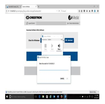
5. Press the Start and Stop button to start or stop sharing to the display in the room.
