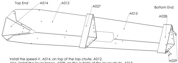
Also, install the lower brace, A028, on the outside of the lower chute, A013.
