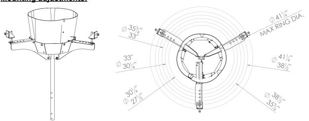
Depending on Grain Bin configuration, you may need to cut off excess bracket, especially in bins with smaller bin lid openings.
