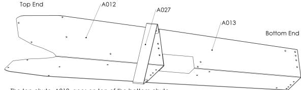
The top chute, A012, goes on top of the bottom chute, A013. Install brace A027 on the inside of both chute members. Round bolt heads go inside. Tighten. For 50/50T/55 models, substitute L001 for A012 and L002 for A013.
