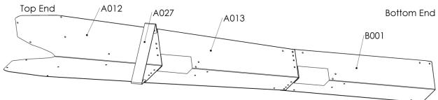
For the 200/200T/250 model, install additional lower chute extension, B001.
