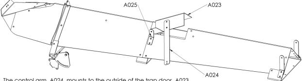
The control arm, A024, mounts to the outside of the trap door, A023.
