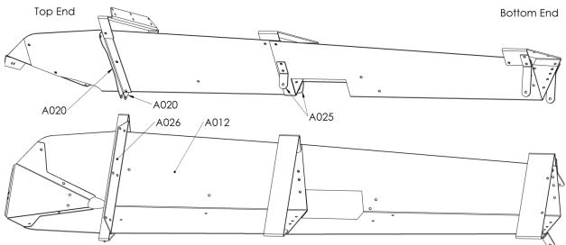
Install the trap door ears, (2) A025, to the v-chutes as shown above. Install the angle iron bracing, (2) A020, on the underside of A012, near the to pend. Then install the adjustment mount bracket, A026 on the ouside of the angle iron bracing, A020.
