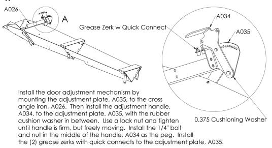
For the 200/200T/250 model, there will be a second handle, A034, for controlling the second trap door. It will need installed on the opposite side of the adjustment plate, A035. Again, use the rubber cushion washer in between the handle and plate and tighten with lock nut until firm, but still freely moving.
