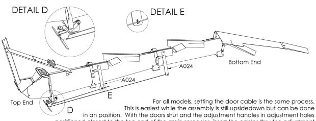
positiioned closest to the top end of the grain spreader, insert the cables thru the adjustment handle holes that are closest to the bottom end and then pull tight down to the trap doors control arm. Use the provied cable clamp inserted through the 2 holes on the control arm to secure the cable in this position.
