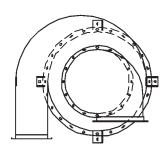
**RC Series Cyclones** are typically used as primary receivers for dry bulk solids in our pneumatic conveying systems.
