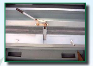
Front View - with machine power locked out, hinged door opened and cylinder cleaning system disengaged.
