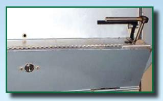
Front View - showing use of existing hinged door with safety latches - inspection doors closed.
