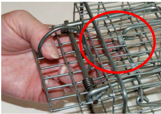
Step 2: Holding door to top of trap, pull pan trigger hook forward to hold door in the up position. Trigger hook can be adjusted for light or heavy set by shifting position of hook as it rests on door.
