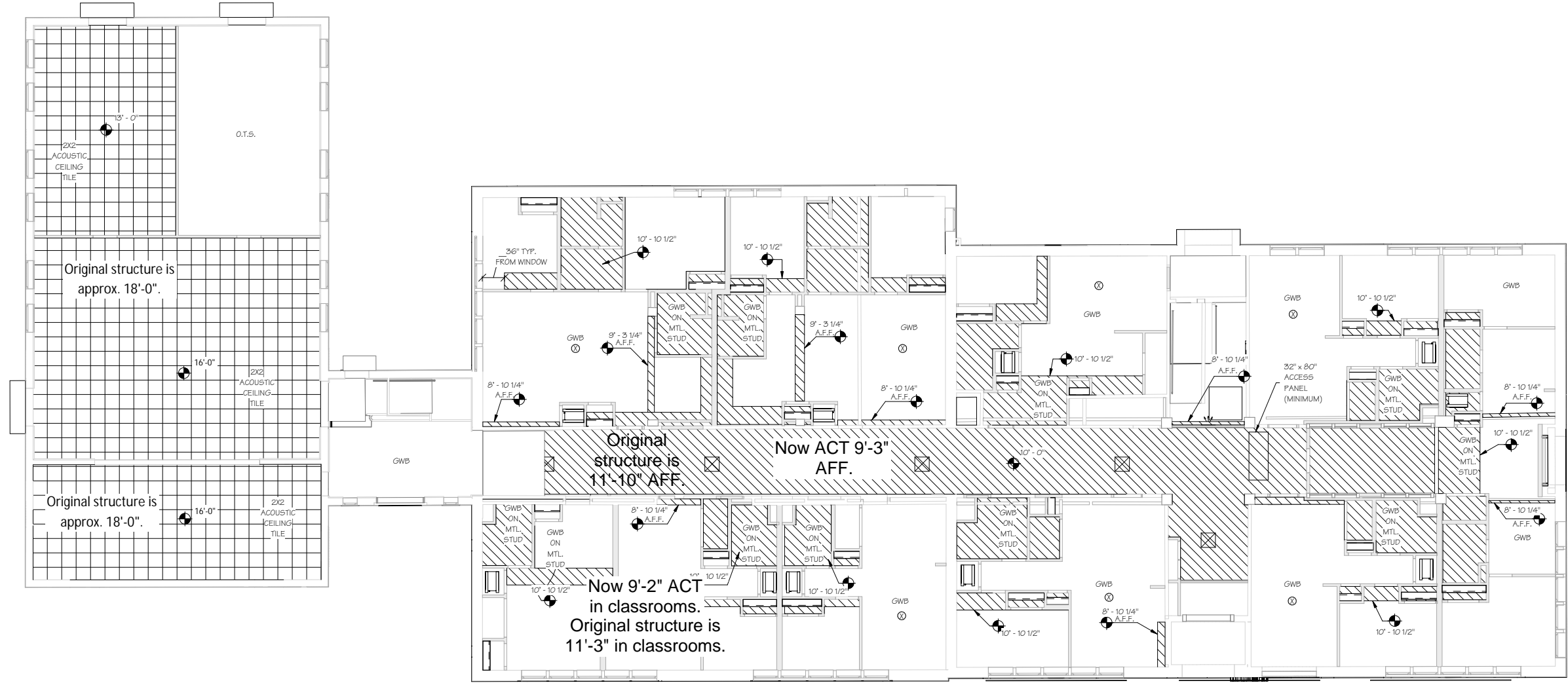
FIRST FLOOR RENOVATED REFLECTED CEILING PLAN
